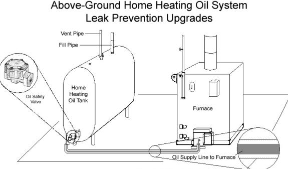
Upgraded Oil Supply Line Protective Sleeve
